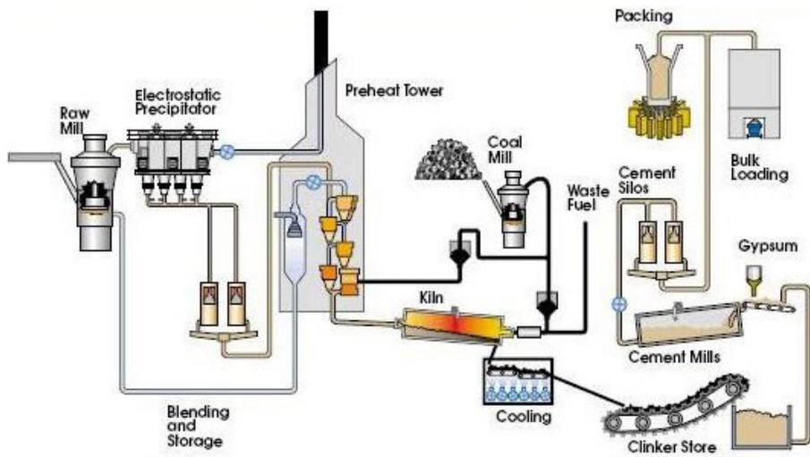
Figure 1. Cement production process.
