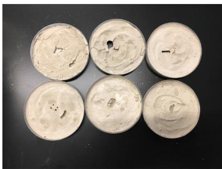
**Figure 4. Basalt and calcium oxide samples of varying ratios. Percent calcium oxide for top row left to right: 25%, 20%, 15%. Bottom row left to right: 10%, 10%, 5%.**
