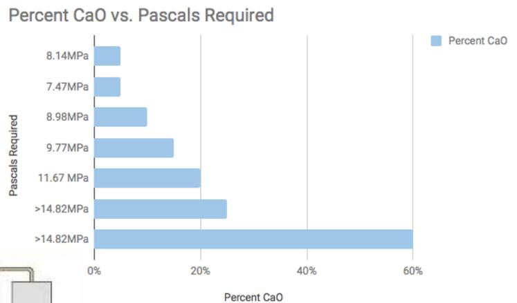
Figure 3. Relationship between the percentage of calcium oxide and the Pascals required to break the cement.
