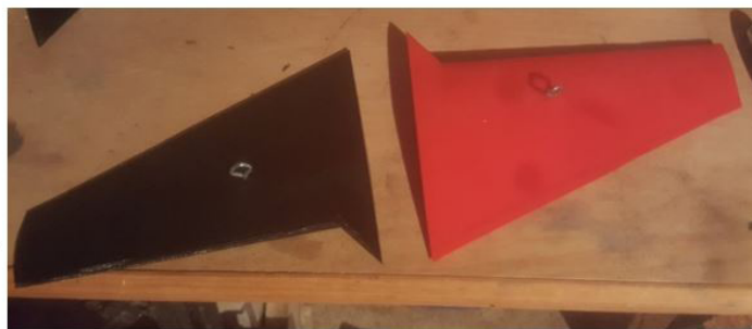
Figure 5: Depicts the comparison between rear (black) and forward (red) swept models.
