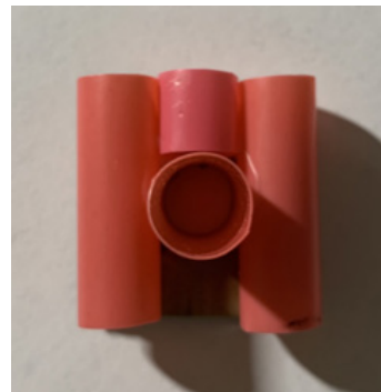
Figure 3: The shaft and the arrangement of the bubble tea straws used for support.
