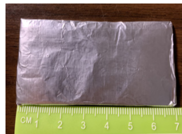
Figure 22: The dimensions (7 x 3.8 cm) of the second piece of cardboard covered foil.
