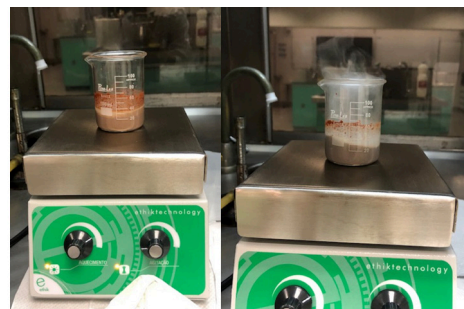
Figure 7: Red mud in a magnetic stirrer being heated.
