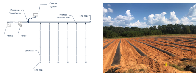
Figure 2: Basic schematic of drip irrigation system.
