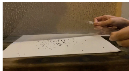
Figure 10: Control group: The microplastics were not attracted to the uncharged acetate.
