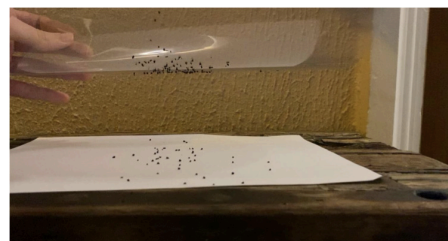
Figure 11: Experimental group: The microplastics were attracted to the charged acetate.
