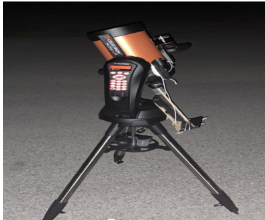
Figure 2: Image of telescope with the spectrometer attached.
