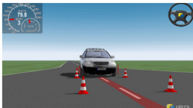
Figure 10: Simulation test for DLC.
