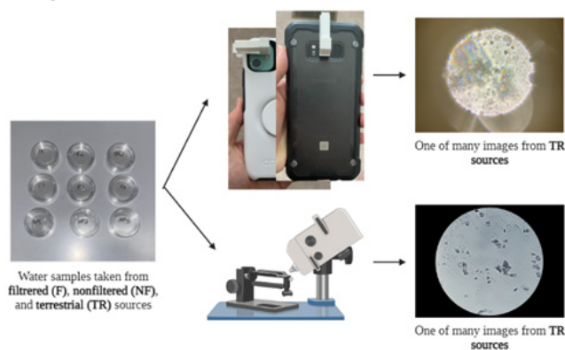
Figure 5: This schematic demonstrates our testing comparisons between PuriScan and conventional microscope methods of filtered (F), nonfiltered (NF), and terrestrial (TR) water sources. Since PuriScan scans on a 350x magnification, the bacteria can be more clearly seen in PuriScan compared to the microscope (on 250x magnification).
