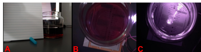
Figure 11: (A) Materials used for the experiment. (B) The card beneath the wine sample is not visible when illuminated with white light (or visible light). (C) The card beneath the wine sample is distinctly visible when illuminated with NIR light and the wine sample also appears clear (since NIR light was not absorbed by wine).
