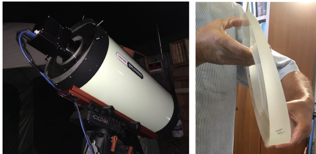
Figure 1: All observations were made using a RASA Schmidt telescope with a prism over the front (at left). The wedge prism was custom-made and has a 7-degree angle (right image). The faces are polished flat to within 1 wavelength of visible light. The flint-type glass, with its large refractive index, spreads the incoming light into all optical wavelengths. 11
