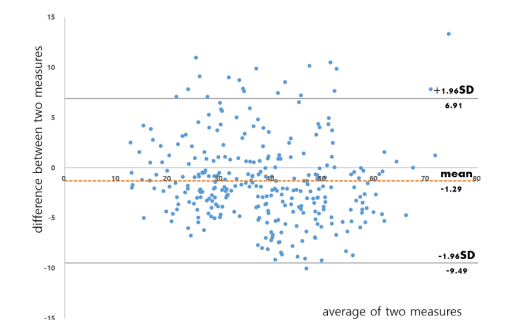
Figure 3: Bland-Altman plots between the Cobb angle measurement by experts and those by the proposed method. The graph shows no specific pattern, with a mean difference of -1.29 and 95% limits of agreement ranging from -9.49 to 6.91.
