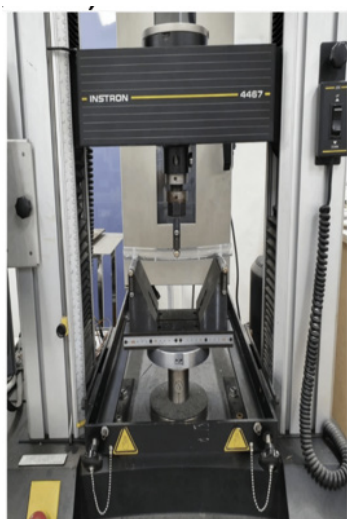
Figure 4: The INSTRON 4467 machine performing the three-point bending test.
