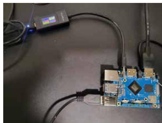
Figure 1: Experiment setup - Orange Pi 5 Pro with Yojack USB power meter.
