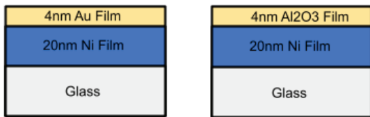
Figure 3: Sample cross sections of Au and \text{Al}_2\text{O}_3 -capped Ni. Both comprise a 20nm Ni film layer on a glass substrate, capped with a 4nm layer of Au and \text{Al}_2\text{O}_3 , respectively.
