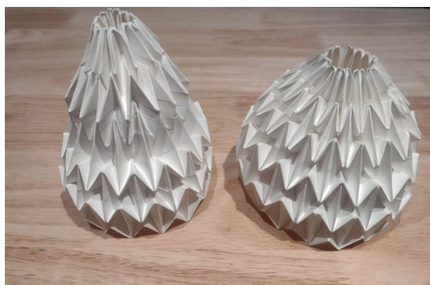
Figure 2: Folded Origami Skeletons; The combined Miura-ori Waterbomb pattern (left) consists of a Miura-ori upper portion and a Waterbomb “magic-ball” lower portion; The Waterbomb pattern (right) consists of a Waterbomb “magic-ball” pattern.
