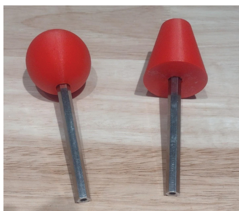
Figure 6: Gripping Objects: Sphere (left) and Frustum (right) connected to hex shafts to fix to Tinius Olsen 25 ST Universal Load Tester. A frustum shape with a wider base at the bottom than the top was tested to assess the combined Miura-ori Waterbomb pattern gripping adaptability improvements.
