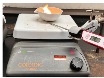
Figure 18: Flash point testing experimental setup and results. This shows the stability of the biodiesel and whether it meets the ASTM limit.
