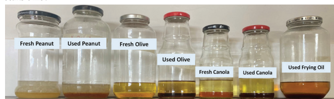
Figure 1: Biodiesels are produced from used cooking oils. The feedstock used to create each biodiesel is specified on labels on the jars. The top visible layer is the biodiesel, and the bottom visible layer is the glycerin.
