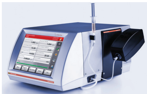
Figure 16: Image of a viscometer, an instrument used to measure viscosity.
