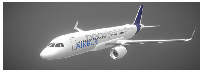
Figure 3: Rendering of Airbus A320-200 NEO. An incremental development aircraft part of the A320 aircraft family. This aircraft is fitted with next-generation engines, improving the aircraft's fuel efficiency.
