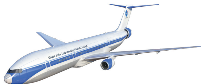
Figure 2: Simulation render of the STARC-ABL configuration. An aft-mounted electric BLI propulsor (powered by the podded engines) ingests the boundary layer air.
