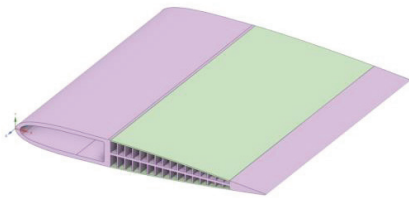
Figure 3: FishBAC 90° configuration isometric view taken on ANSYS SpaceClaim.
