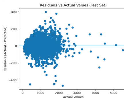
Figure 7: Residuals vs actual scatter plot. Each dot is a model prediction on the test set, with the 0 line indicating a perfect prediction. Dots above and below the line represent overpredictions and underpredictions, respectively. Randomly scattered dots above indicate that the model is not systematically biased towards any range.
