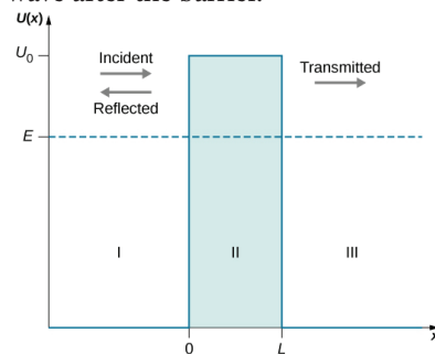
Figure 1: The visualization of quantum tunneling. Adapted from Physics LibreTexts. 4 This figure shows that even when the particle's energy is below the barrier height, part of the wavefunction can extend through the barrier and produce a transmitted wave.
