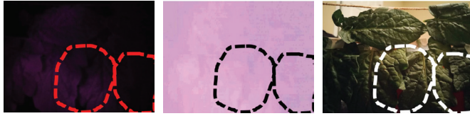
Figure 2: NIR photons were detected by a cell phone camera, which generated the NIR images. There are two tomatoes fully hidden behind leaves in both the left and right images. The image on the left is the raw image, in which the fully hidden fruits cannot be seen. The center image shows the image after the PLIA preprocessing. The image on the far right is the corresponding RGB view of the other two images. Dotted lines on those images delineate the approximate locations of the two hidden tomatoes.
