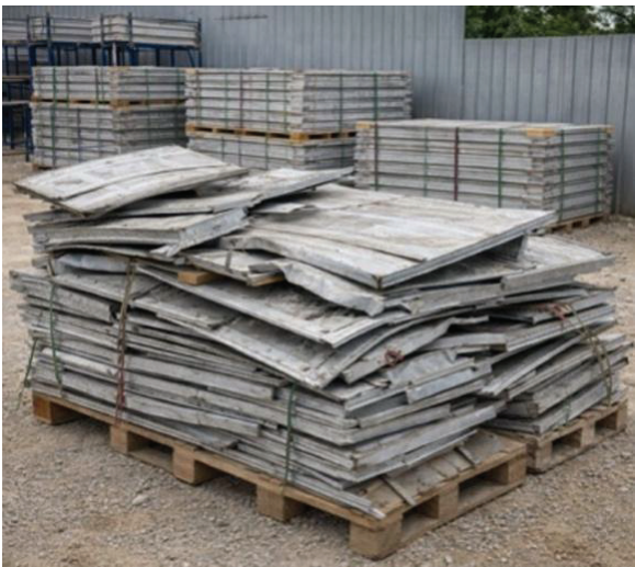
Figure 10: The damaged panel during de-shuttering was caused by improper handling.
