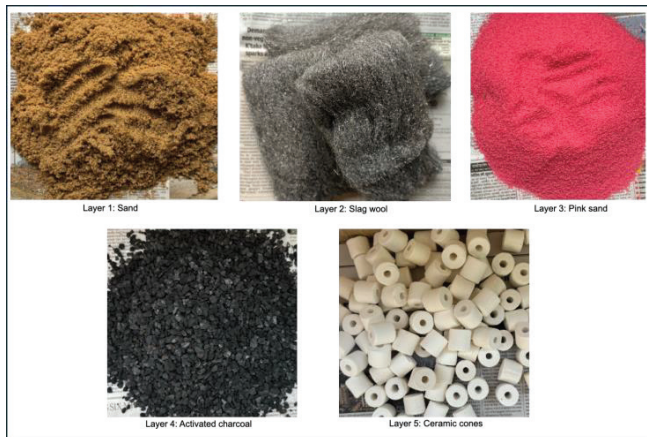
Figure 4: Materials used in the filtration column for water purification. Layers of coarse sand, slag wool, pink sand, activated charcoal, and ceramic cones, available in bulk locally in all environments, were chosen for further experimentation.
