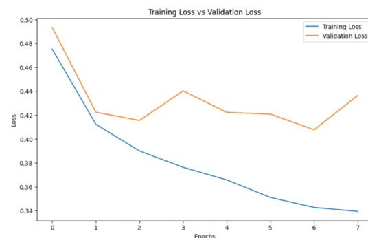
Figure 5: Displays the training vs. validation loss across multiple epochs. Training loss is depicted as consistently decreasing toward zero. Validation loss, on the other hand, plateaus around 0.42 to 0.44, indicating clear overfitting within the Bi-LSTM model.
