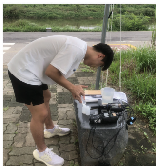
Figure 8: Part of a field sampling and in-situ measurement (pH, Temp., DO, Eh, EC, and alkalinity).
