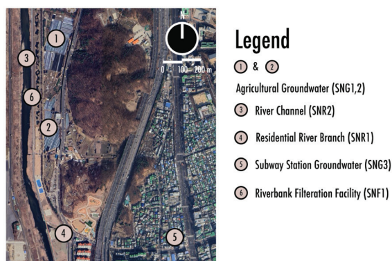
Figure 7: Spatial distribution of sampling and monitoring points in the study area, including agricultural groundwater wells (SNG1, SNG2), river channel (SNR2), residential river branch (SNR1), subway station groundwater (SNG3), and riverbank filtration facility (SNF1), all situated in proximity to the main and tributary streams.
