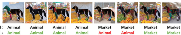
Figure 4: Example results of the proposed method. The model incorrectly classifies later Market images as Animal images because it saw Animal images first. This demonstrates that the network reproduces perceptual hysteresis, exhibiting prediction biases that depend on the sequence of preceding frames.
