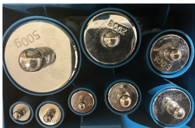
Figure 11: Weights kit including weights of 10g, 20g, 20g, 50g, 100g, 100g, 200g, 500g, totalling 1 kg overall.
