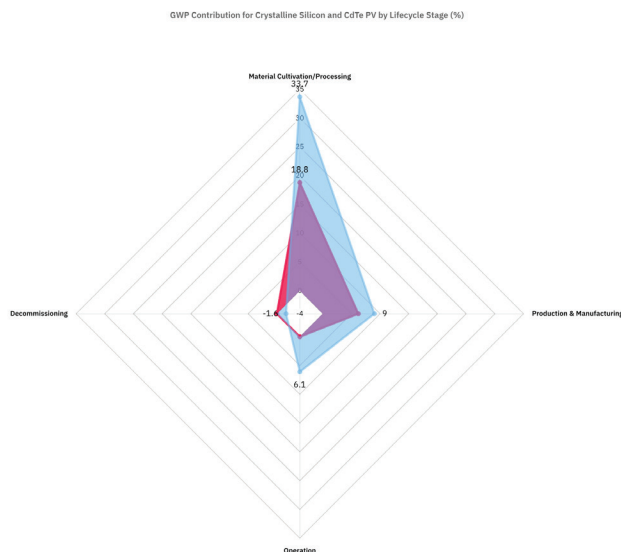
Figure 1: GWP contribution for crystalline silicon and CdTe PV by life-cycle stage (%). This radar chart compares the GWP breakdown for first-generation crystalline silicon (blue) and second-generation CdTe thin-film (red) solar PV. The distance from the center along each axis represents the percentage contribution of that stage to the total GWP. For example, Material Cultivation/Processing accounts for 33.7% of the GWP for crystalline silicon. Negative values, such as those for decommissioning, represent environmental credits from recycling that offset a portion of the emissions. The data shows that material cultivation and processing represent the largest GWP contribution for both technologies, especially for crystalline silicon. This highlights how the energy intensity of early stages, rather than manufacturing or operation, is the largest contributor to solar PV's carbon footprint. Data synthesized from Nugent & Sovacool (2014). 8
