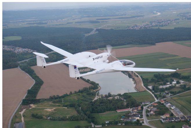
Figure 4: The HY4 aircraft in flight using liquid hydrogen. Source: H2FLY.
