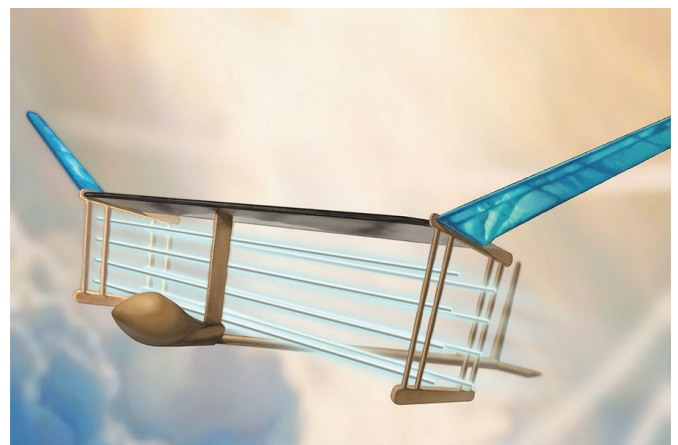
Figure 1: Rendering of MIT's ionic wind aircraft demonstrating electrohydrodynamic propulsion. Source: MIT News, Christine Y. He.
