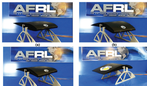
Figure 4: The morphing airfoil design by FlexSys Inc. being researched at the U.S. Air Force Research Laboratory, showing the capabilities of shape memory alloys in airfoil profile change. 17
