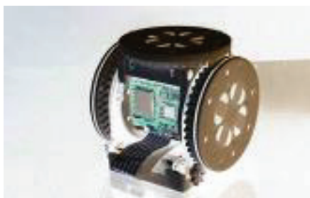
Figure 3: Anibot modules visual. Combined, this module functions as a flexible modular robot. 13
