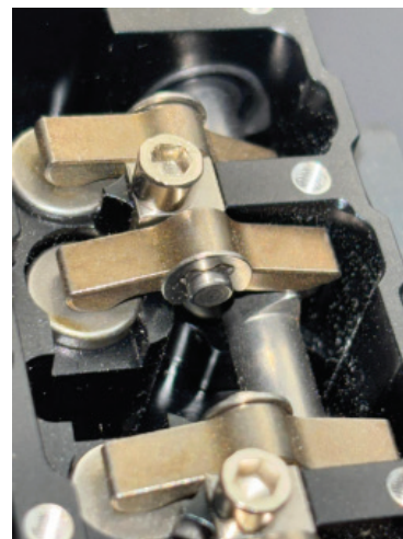
Figure 6: Camshaft from a SEMTO ST-NF2 Inline Twin Cylinder Engine Model. Demonstration of the camshaft mechanism.
